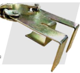
The unique way in which the Toe Board is held away from the standard has led to the adoption of the Tamer with various types of system scaffolding, as it allows traditional timber scaffold boards to be used as Toe Boards without fouling the ring or cup. When using scaffold boards to form the working platform on the above systems, the Tamer unifies the platform in a way that was unattainable previously.
